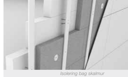
Isolering bag skalmur
